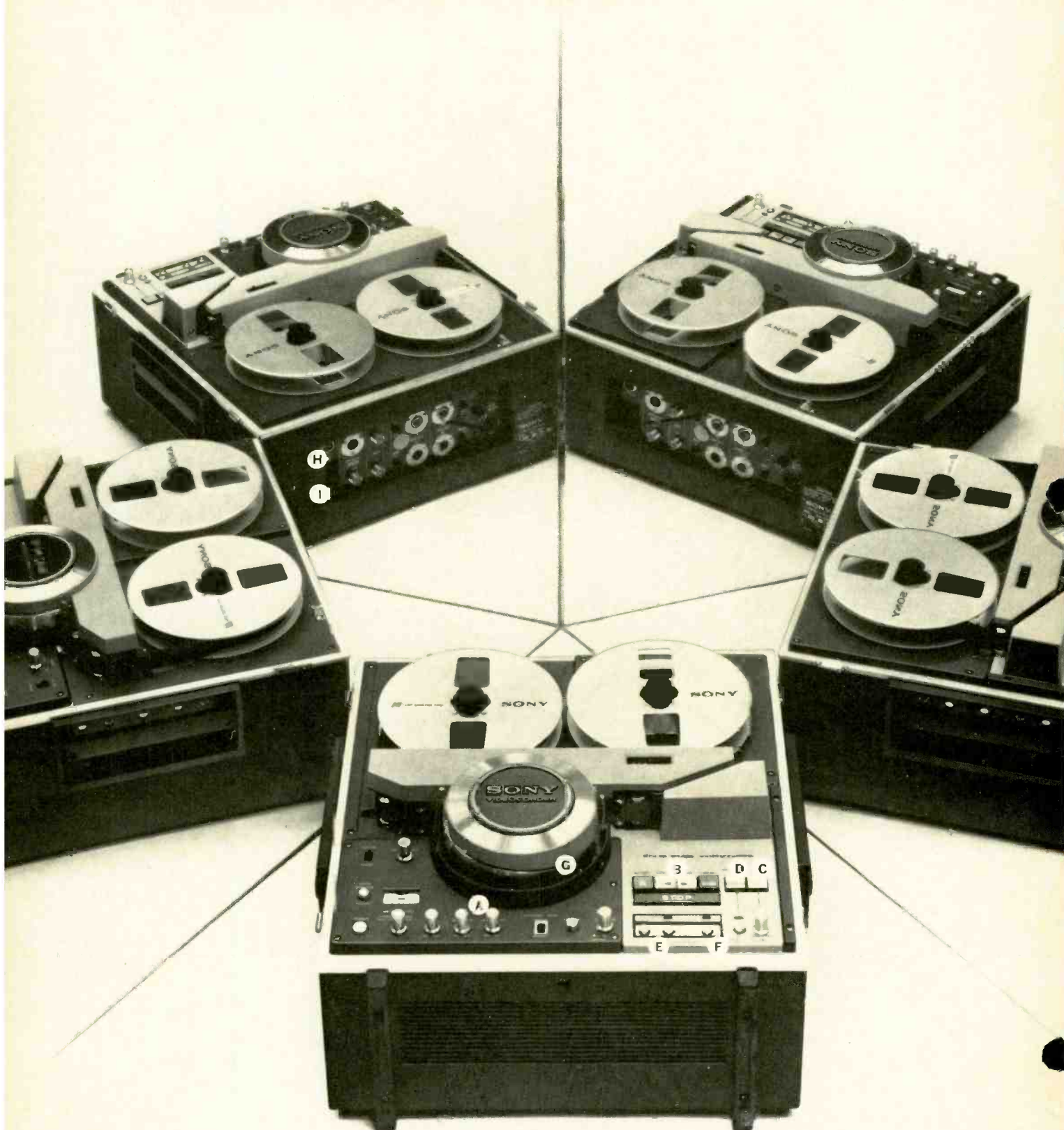
A. TWO INDEPENDENTLY CONTROLLED AUDIO CHANNELS B. SOLENOID-OPERATED PUSHBUTTON CONTROLS C. VARIABLE SLOW SPEED/STILL CONTROL D. AUDIO CHANNEL 2 DUBBING E. VIDEO SIGNAL INSERT (CUT IN & CUT OUT) F. VIDEO SIGNAL ASSEMBLY G. ROTARY ERASE HEAD H. COLOR ADAPTER CONNECTOR I. REMOTE CONTROL CONNECTOR
