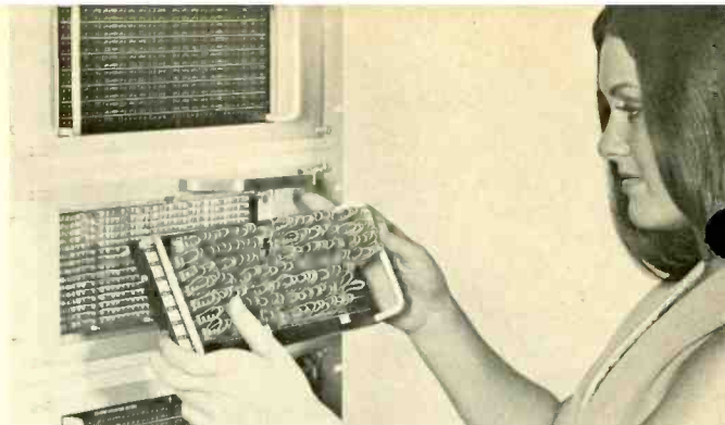
Flexible intercom system uses preset patch panels which can connect any desired calling station with any listening station.
