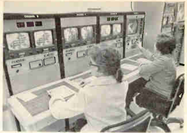
Line/Preview console (LPC) operators, Barbara Bromley (left) and Judy Deal, monitoring on-air programs of four channels.
