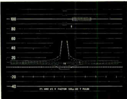
Fig. 1. The Tektronix sine 2 K-factor graticule. Two sweep speeds are provided on these waveform monitors so that this graticule can be used for 0.125 \mu s T-pulse testing on such applications as studio and network transmission lines, and for 0.250 \mu s 2T-pulse testing on such applications as video tape recorders and transmitters.
