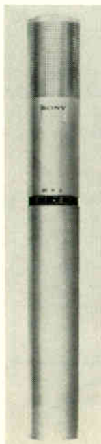
Economy condenser microphone from Sony (far left), the model C-22 is tagged at $99.50. It has usable response to 20 kHz and cardioid pickup pattern. FET preamp is self-contained, as is battery supply. (Below, left) Guts of updated old-standby Neumann condenser U87i, show compact FET transistor preamp. Self-contained battery supply is on reverse side. Mike has selectable polar patterns and almost ruler-flat response (see curve on p. 37). AKG's modular mike (below, right) has screw-on condenser head, modular preamp in the tube, and add-on accessories for extra versatility such as shotgun mike applications.
