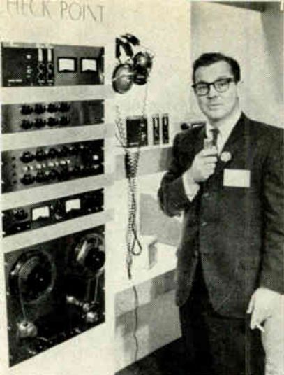
Budget-priced mixer and control line by Gately (left) provides flexible console designs. Neumann condenser mike (above) and cigarette-pack-size preamp/power supply were part of star performer line showed by Gotham Audio. One of line of Vega wireless microphones (right), transmitter pack is built into extension of Shure microphone case, and trails wire antenna. Line offers mike flexibility.
