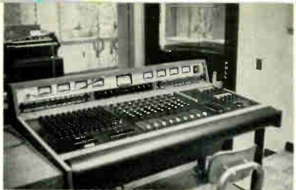
BM/E Photo Eight-channel console in Studio 2's control room is largely custom-built by Mercury engineers.
