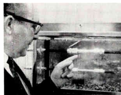
Trenching and cable burying equipment was shown by Davis (top photo) and Sod Master. AMP-Fit one-piece molded nylon fitting by AMP, Inc., (center photo) is rated at 300 lb/in 2 , crimps onto metal or plastic tubing. (Bottom) Hermetic seal of Gilbert coax connectors is demonstrated by display in water-filled aquarium.
