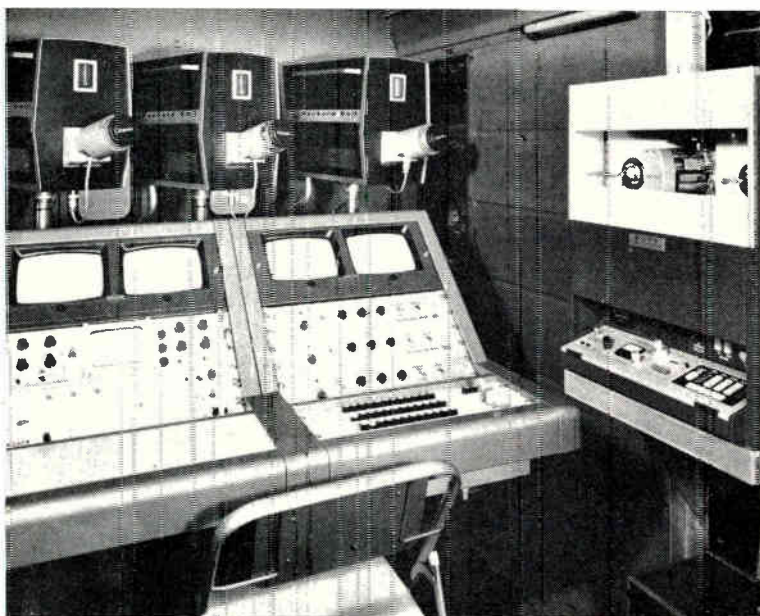
Packed for travel (above), van stores its three Packard Bell cameras above console. (Right) Van is compact, unobtrusive.
