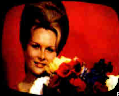
Off-the-monitor photos demonstrate excellent color quality and sensitivity of 3-vidicon design. Lighting levels above: (A) studio light at less than 150 ft. candles, (B) studio light at 300 ft. candles, (C) outdoor lighting at 4,000 ft. candles.
