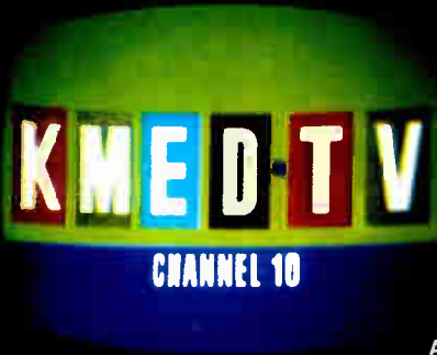
Off-the-monitor photos demonstrate excellent color quality and sensitivity of 3-vidicon design. Lighting levels above: (A) studio light at less than 150 ft. candles, (B) studio light at 300 ft. candles, (C) outdoor lighting at 4,000 ft. candles.
