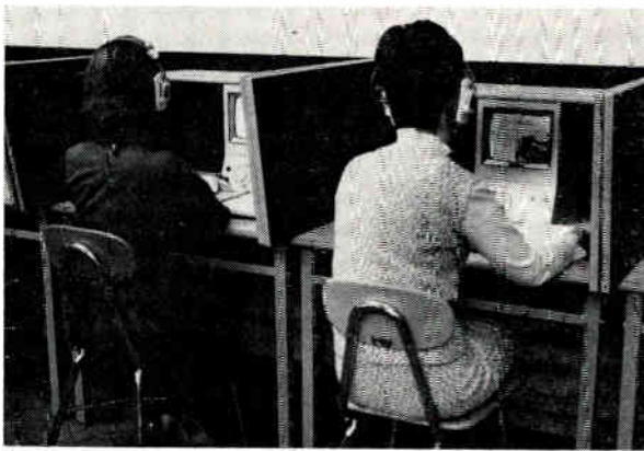
Carrel with dial retrieval system which can select a portion of a videotape at Burnt Hills.
