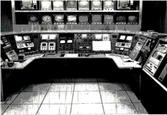
Master control console for two station outputs. WMVT switcher on left, WMVS switcher on right, camera and film controls in center. Color control console (lower right) incomplete. Line and preview monitors in rear monitor rack.
