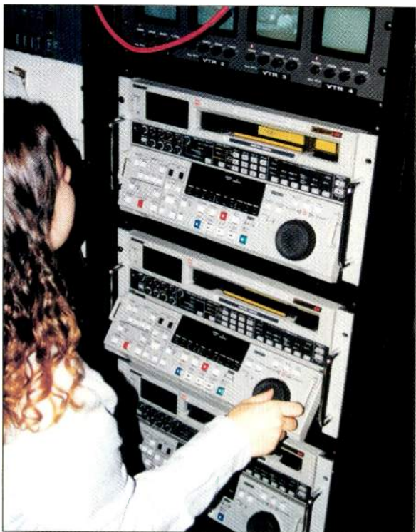
CT-N uses Sony Betacam SX decks for multiple sequential recording.
