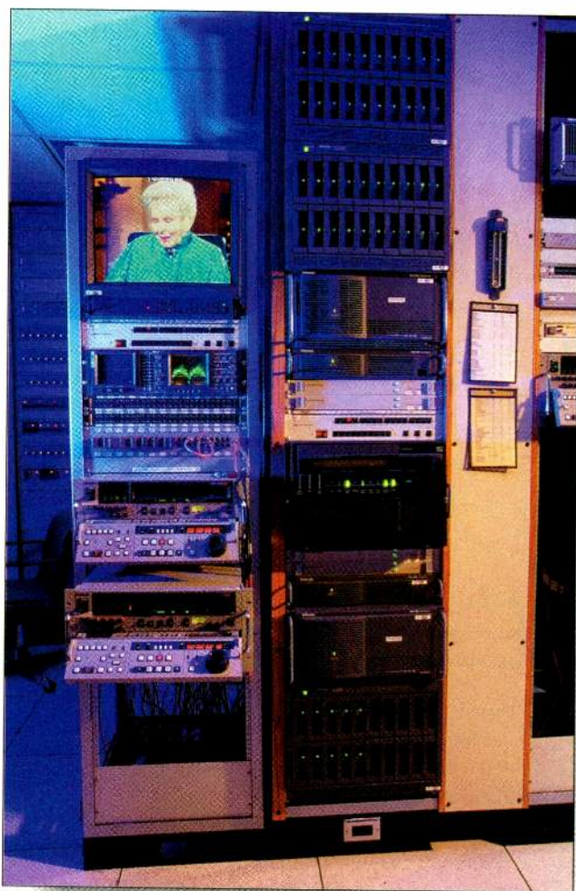
Video servers using MPEG compression are now found side-by-side with tape machines in broadcast facilities such as KOMO-TV. Photo courtesy Grass Valley Group.
