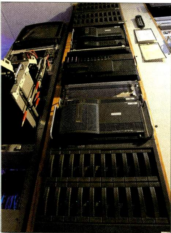
Compression has made the use of disk storage and playback systems, such as these video servers at KOMO-TV, cost-effective. Photo courtesy Grass Valley Group.
