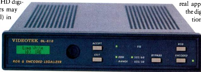
The DL-810 Serial Digital Legalizer evaluates 601 video in real time on a pixel-by-pixel basis and provides an output guaranteed within NTSC or PAL encoded legal limits.
