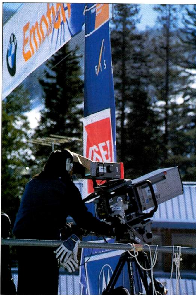
Today's cameras are expected to operate under a wide variety of conditions, including weather extremes. This Philips LDK23 high-speed, ultra-slow motion camera was used at the 1999 World Alpine Downhill Ski Championship in Aspen, CO. Photo courtesy Philips.
