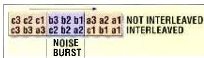
Figure 2. Simplified illustration of data interleaving. A noise burst that obliterates all three "B" bytes of a non-interleaved signal, covers only a single A, B and C byte of an interleaved signal. This leaves enough data for the Reed-Soloman decoder to determine the correct values of the missing bytes.
