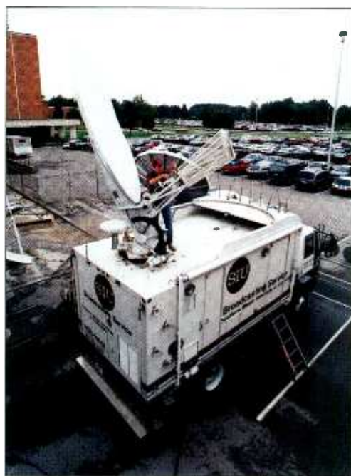
Due to increased stress from vibration and weather extremes, mobile uplinks require frequent inspection and lubrication of mechanical components. (Photo courtesy of Southern Illinois University Broadcasting Service, Carbondale, IL.)
