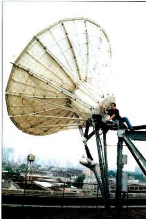
For the safety of those involved, always remove power from the drive motors before starting any maintenance.
