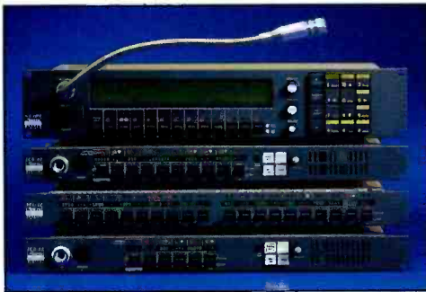
From the top, a 12-key LCD display station, a 9-key LED display station, a 20-key LED expansion panel, and a 5-key LED display station.
