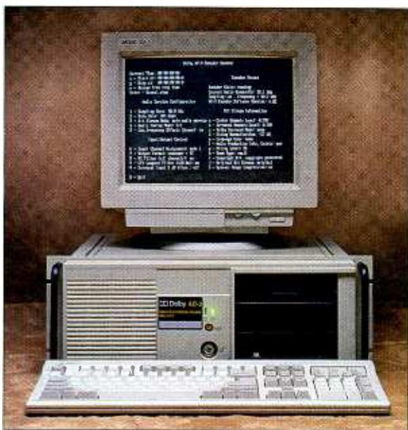
The Dolby DP561 is a PC-based encoder for the AC-3 multichannel digital audio data-compression algorithm.
