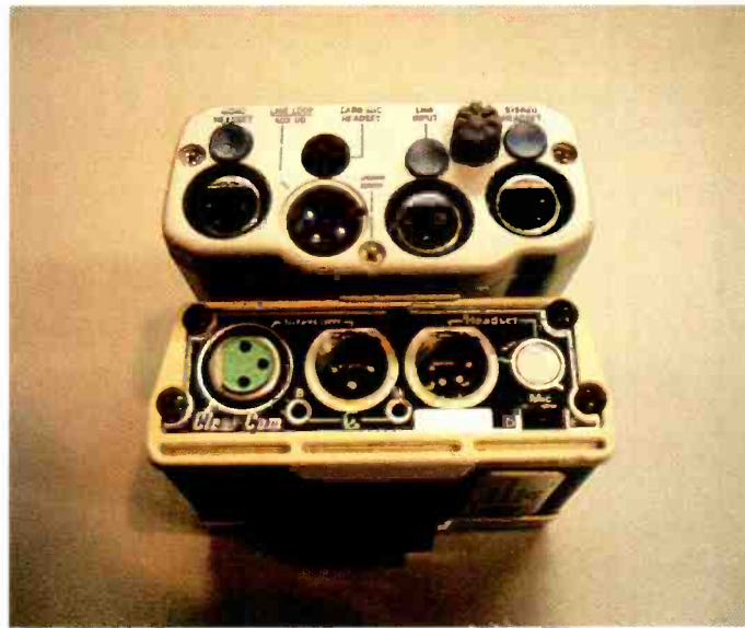
The beltpacks of two popular intercom systems, RTS/Telex (top) and Clearcom, use the same connectors and cables for the same functions, but their systems are not compatible.
