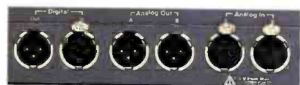
Input and output ports allow you to generate test signals for both analog and digital domains.
