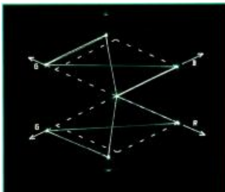
Figure 3. Excess level in the green channel moves the trace beyond the graticule in both diamonds. Note red
