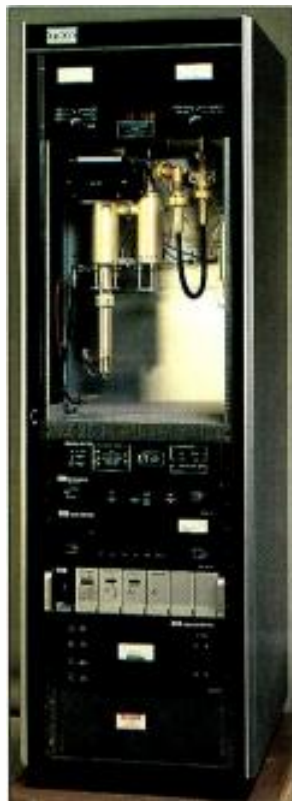
The EMCEE TTU1000E, a 1kW UHF tetrode transmitter, the translator version is the TU1000E.
