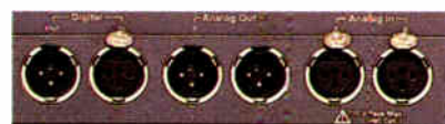
Input and output ports allow you to generate test signals for both analog and digital domains.
