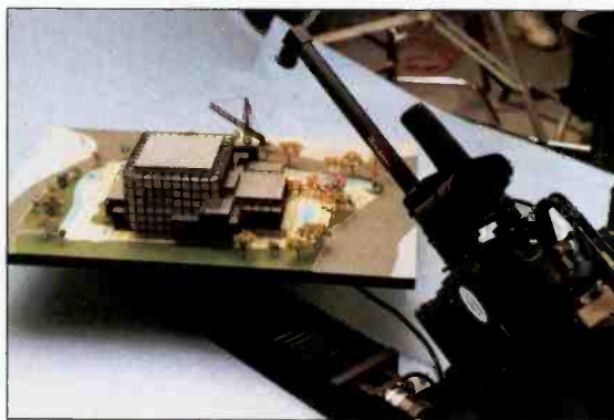
The camera and motorized table setup used to shoot miniature models. (Photo courtesy of Innovision.)
