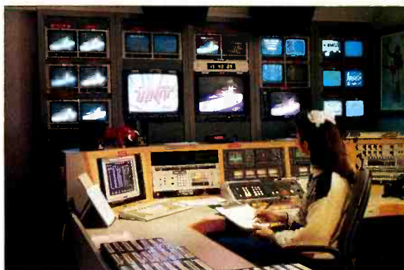
The master control area at TNT Latin America. Operation is semi-automated, with VTRs under the control of the cart machine.
