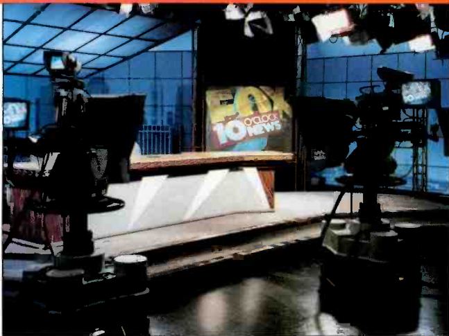
Two recently installed robotic camera pedestals on the news set of WNYW, New York. (Photo courtesy of AF Associates.)
