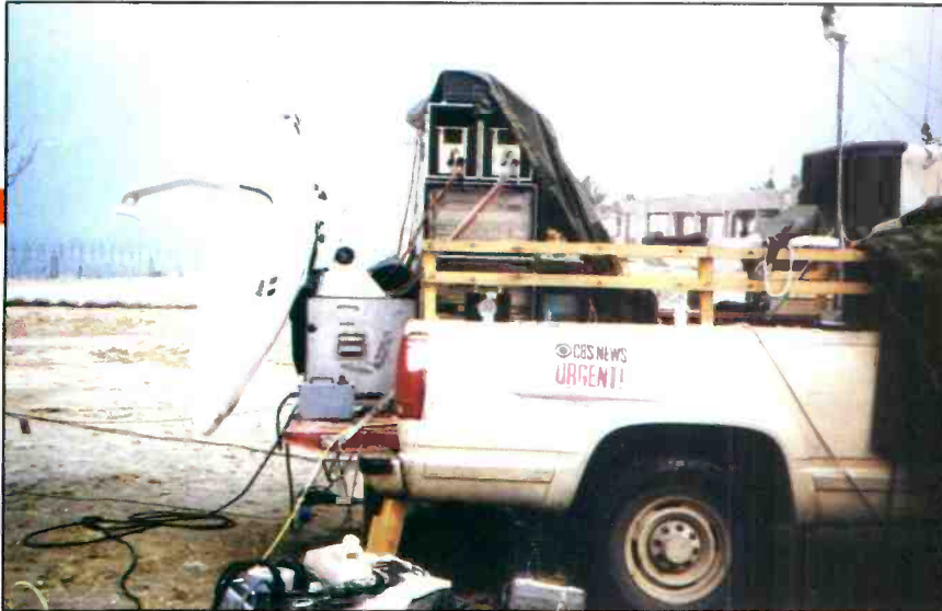
The uplink dish used by the CBS SNG crew sits on the back of its pickup truck on Feb. 27, the morning after the liberation of Kuwait City. The look angle to the satellite was only 7°. (Photographer: Ed Jackson, CBS News.)
