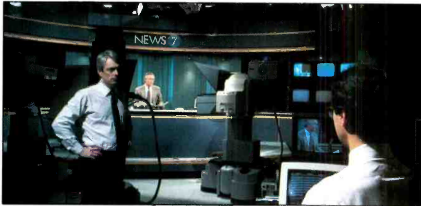
A modern robotic camera system, such as the one shown here, can provide improved control, while simultaneously reducing operating costs. (Courtesy of WHDH-TV)
