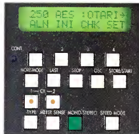
An automatic record and reproduce alignment system drastically reduces set-up time.
