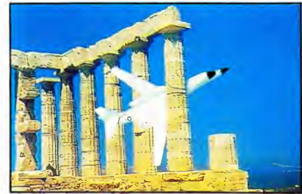
Figure 4. Using a 1-channel ADO effects systems and an AVC Vista switcher with Digi-Loop, the first pillar (background video) is wiped over the airplane key to simulate the jet actually flying through the columns.
