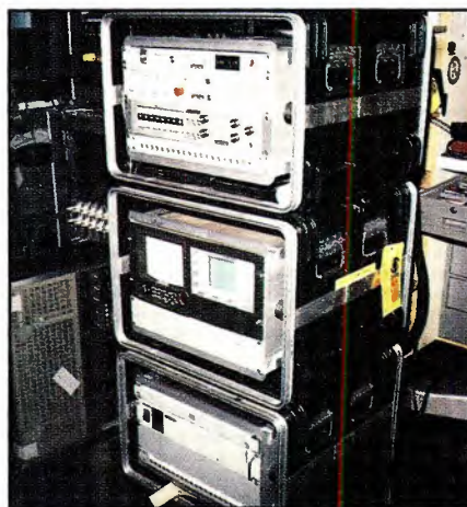
The portable feed pack, which houses audio and video switchers, TBCs, test equipment, signal generators and monitors, has been used since 1982 in the network's modular remote broadcast systems.
