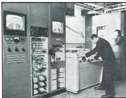
The first broadcast via videotape took place on Nov. 30, 1956. CBS Television City in Hollywood, shown here, replayed the "Douglas Edwards and the News" program three hours after it was received on the West Coast. CBS engineer John Radis stands at the controls of the Ampex VRX-1000. Note the racks of support electronics (on the left) for the tape transport. (Courtesy of Ampex.)
