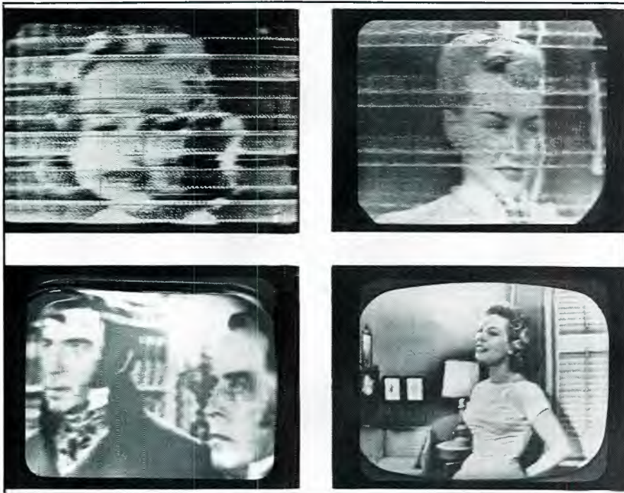
The progress of the videotape recording from 1953 to 1956. Clockwise from top left: Shirley Temple, recorded in late 1953 using AM signal processing; the Bob Crosby show, 1954, using FM signal processing; an FM videotape picture of a kinescope broadcast, mid-1954; and FM recording, early 1956. (Courtesy of Ampex.)
