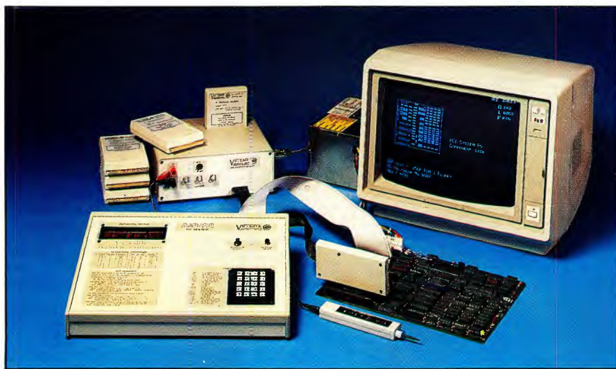
A test unit such as this can apply test signals and interpret results by exercising a computer system through its I/O connections. The system then outputs a message to guide the technician to the suspect pins of the suspect components. (Photo courtesy of Vu-Data Corporation.)
