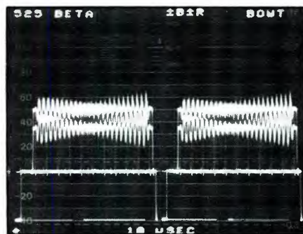
Figure 4. A C-C error will be displayed on a CAV waveform by showing one of the two nulls being off-center.
