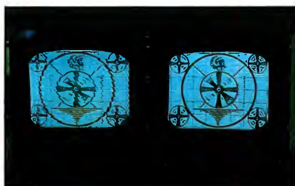
Early VTR engineers constantly had to cope with venetian blinding (shown at left), caused either by inadequate tip penetration or incorrect head spacing (quadrature error). (Courtesy of Ampex.)
