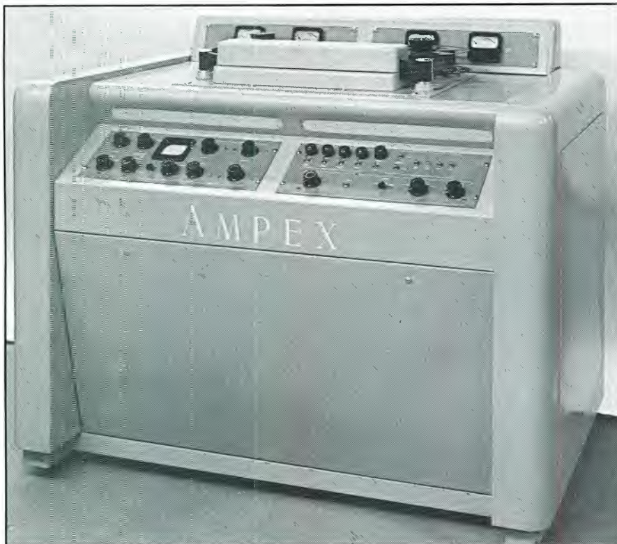
The world's first practical videotape recorder, the Ampex-Mark IV prototype VTR, was unveiled in April 1956 at the National Association of Radio and Television Broadcasters (NAB) convention. (Courtesy of Ampex.)
