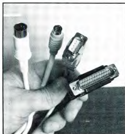
All four of these connectors are used for RS-232, depending on the brand and model of computer. The 25-pin connector (far right) is used most often.
