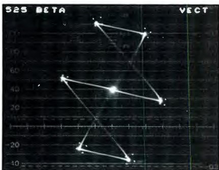
Figure 2. The C-C alignment check using a composite vectorscope. The goal is to adjust the C-C delay so as to place the scope trace between the green dot and the magenta dot so that it passes through the origin.
