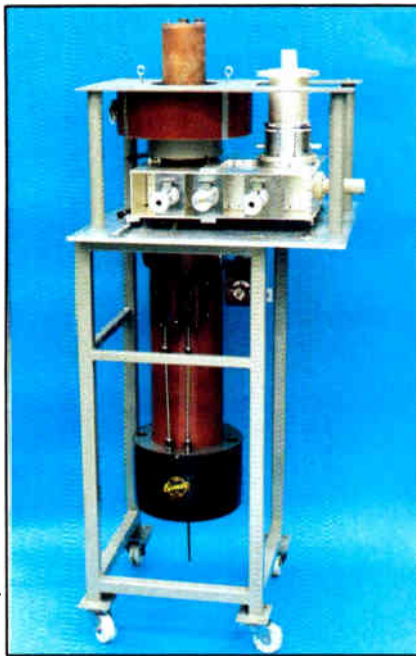
Figure 2. The 60kW Klystrode tube mounted in its support stand with the output cavity attached.
