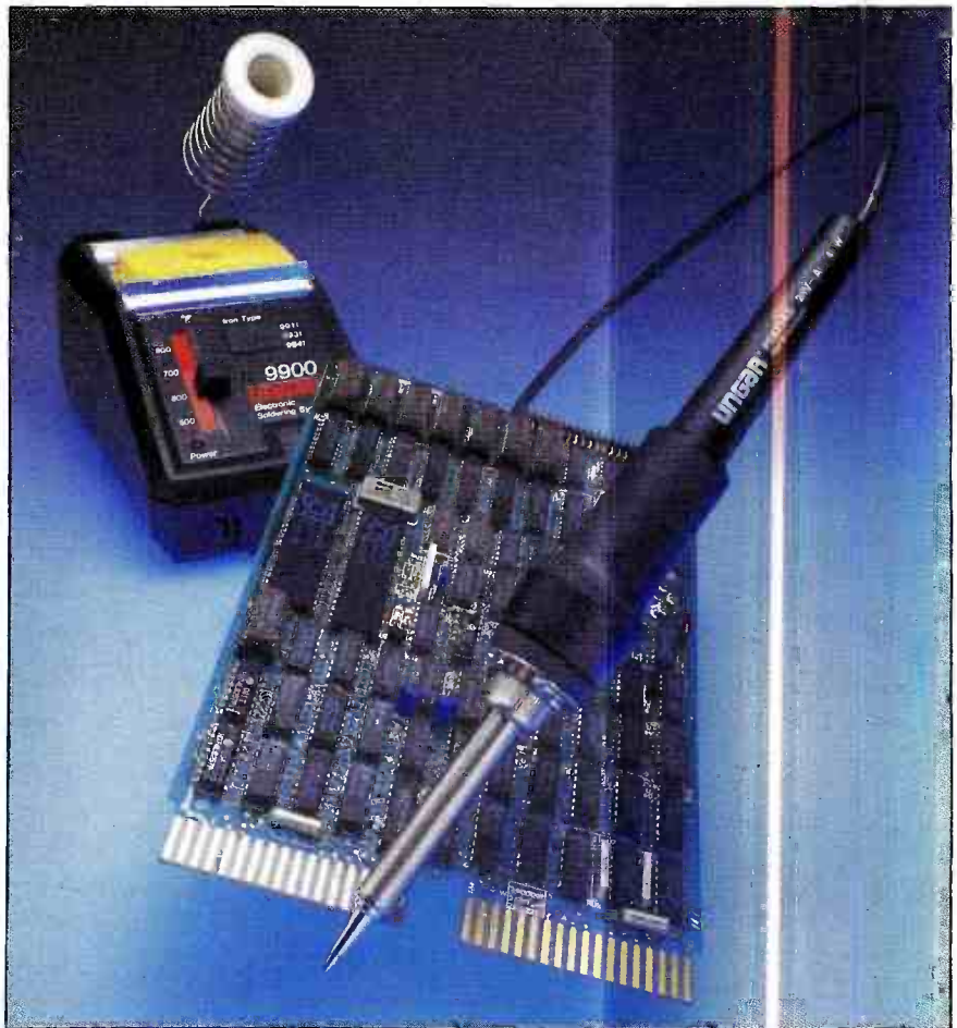
Successful solder rework of a printed circuit board requires skill, patience and the proper tools. One of those tools is a temperature-controlled soldering iron.
