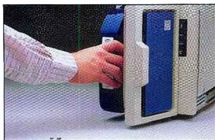
The 825 fixed-media drive can store up to 1,000 stills. Up to 100 stills can be stored on removable disk packs.
