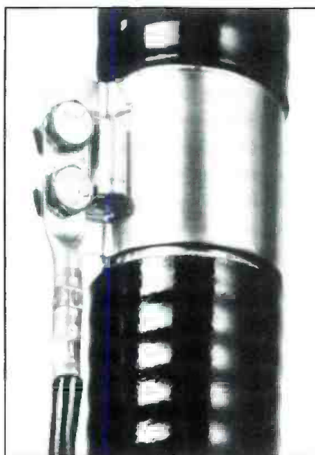
Corrugated cable offers a convenient and effective method of grounding anywhere along the line by stripping the jacketing, attaching a ground strap and covering the connection.
