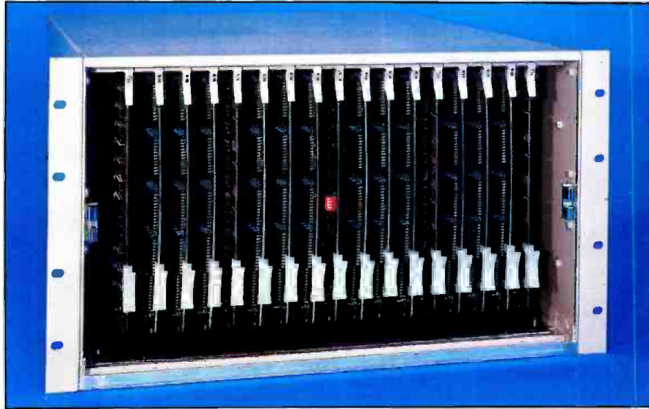
The standard memory shelf of the video recorder. Twelve of the 17 boards in this shelf are used for storing video data.
