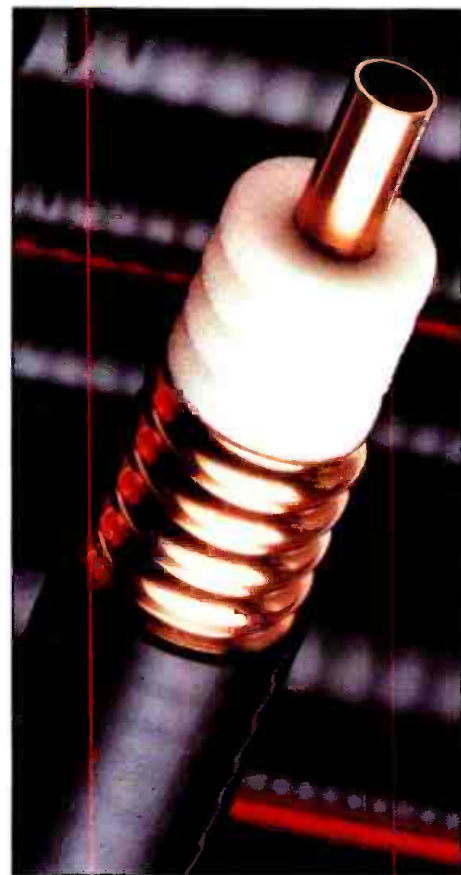
Low-density foam cables are designed to prevent water from penetrating and traveling along the length of the cable. The outer conductor is locked mechanically to the foam dielectric by annular corrugations.
