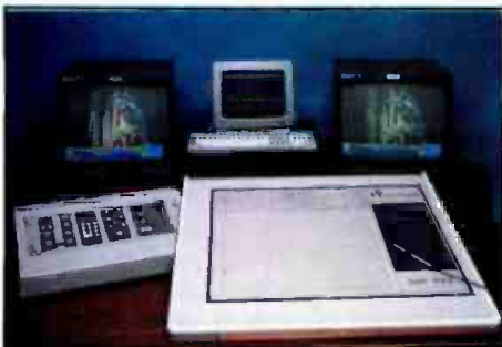
A drawing pad serves as a typical input for the graphics generation function.
