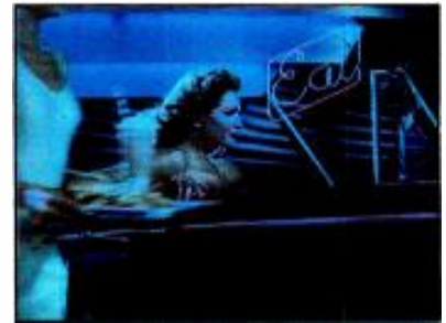
The color grabber allows the colorist to move the screen cursor to any area within the scene. The processor then automatically assigns the appropriate color control to the system. The original yellow dress was changed to white without affecting the scene's colorimetry.
