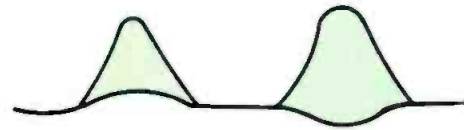
Figure 3. Vertical bowing of the composite baseline indicates amplitude errors. A waveform such as this indicates low B-Y and high R-Y amplitudes.
