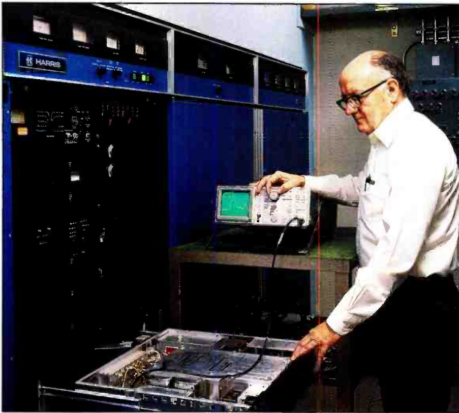
A spectrum analyzer is set to monitor a TV carrier at 196MHz.
