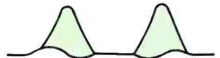
Figure 4. If the composite baseline curves like a sine wave within each pulse, it is because of time delays between Y and color-difference components.
