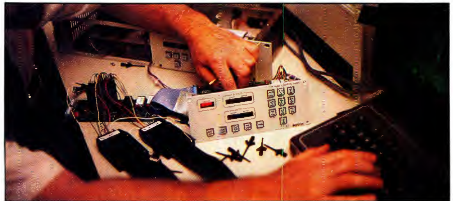
The technician is performing tests with the analyzer. Note the two impedance interface pods that connect the analyzer to the equipment under test.
