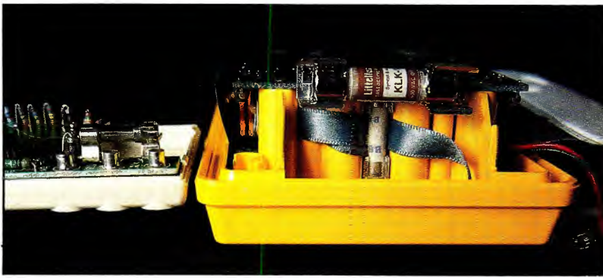
Note the difference in meter protection. The heavy-duty meter has both a 10A and 2A fuse, while the smaller meter has only a 0.8A fuse.
