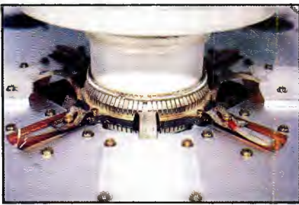
Carefully inspect the PA tube socket assembly. Do not remove the PA tube unless necessary.
