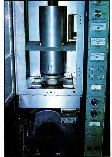
Clean the PA cavity assembly to prevent an accumulation of dust and dirt. Check hardware for tightness.
