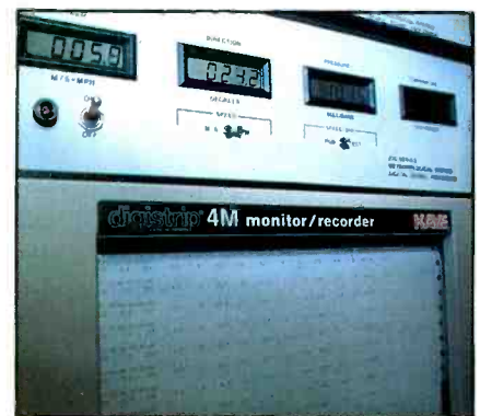
The icing control research package includes meteorological probe readouts, tabular data printer, chart recorder and video recorders.
