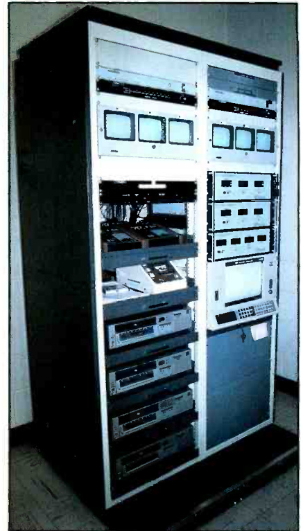
The icing control research package includes meteorological probe readouts, tabular data printer, chart recorder and video recorders.
