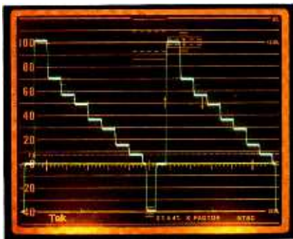
Figure 4. Low-pass filter response with color bars, 2H sweep.
