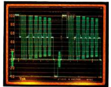
Figure 10. Multiburst signal exhibiting high-frequency rolloff.
