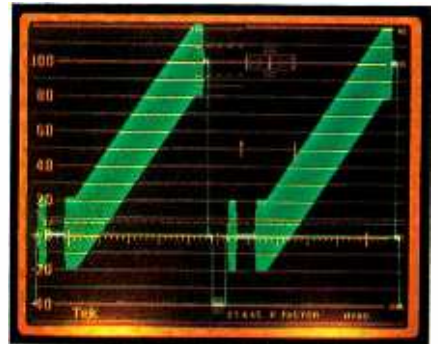
Figure 11. A 100IRE modulated ramp, 2H sweep.
