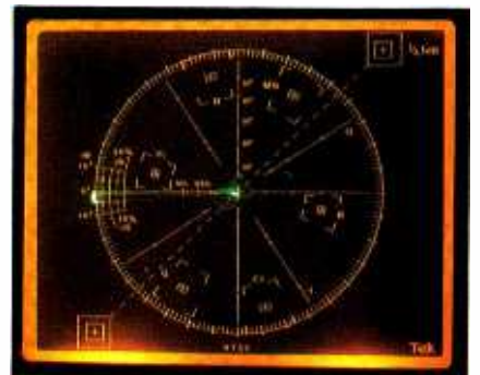
Figure 12. Differential phase of 5° on vectorscope.
