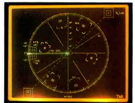
Figure 14. Differential gain of 10% on a vectorscope.
