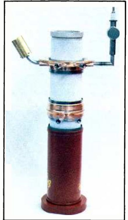
The Klystrode is really a hybrid of the klystron and tetrode.
