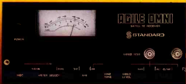
Operating functions including MGC, AGC, AFC, level sets, normal/invert video, clamp/unclamp video, skew, subcarrier frequency selection, video and IF test points are conveniently located on the front panel. Meter reads C/N ratio, signal strength or center-tune.
