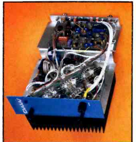
A 600W solid-state VHF module.
