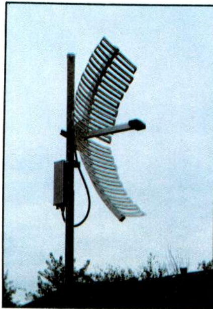
At receiving sites, equipment is simplified to a small antenna with a mast-mounted LNA/receiver. Power is inserted in the VHF RF cable leading to the viewer's set.
