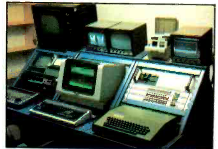
Control for the ITFS equipment includes an automation computer with CRT, keyboard, disk drives and printer. Additional equipment includes monitoring and titling units.
