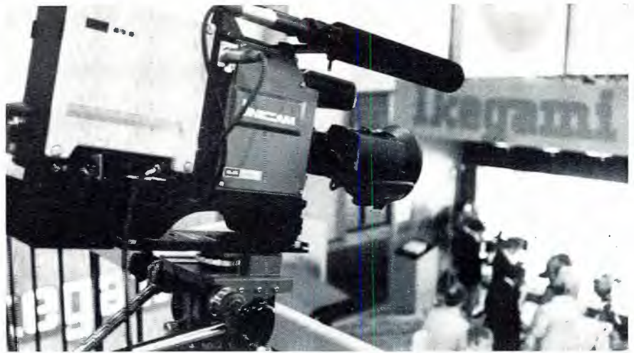
The Ikegami HL-95 camera attaches to a 1/4-inch Hitachi or other format recorders.
