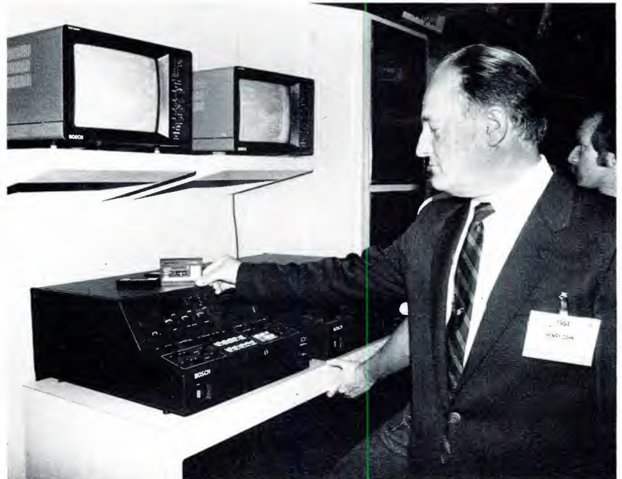
Henry Zahn (Bosch) holds a 20-minute 1/4-inch cassette atop a BCF-9 Lineplex studio recorder.
