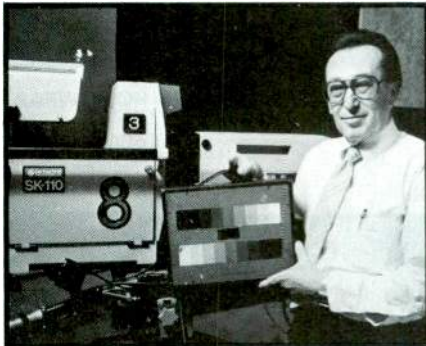
The author with gray-scale setup box he devised. (Note hole in middle of box that creates absolute black reference.)
