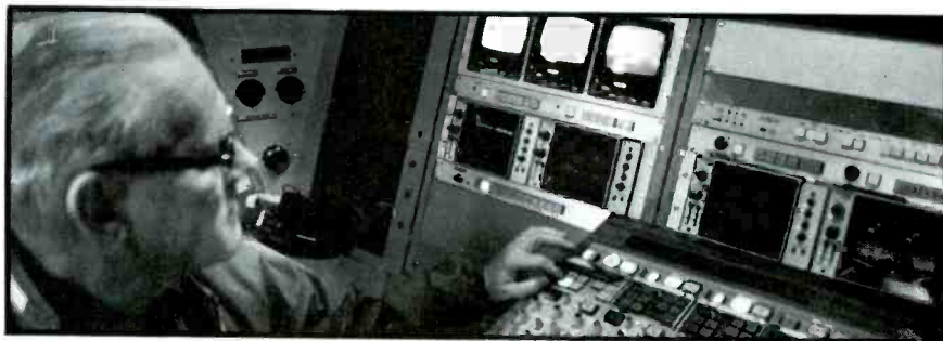
Carl Thompson, master control operator, pushes the button at the RCU to begin the auto setup of one SK-110 camera.
