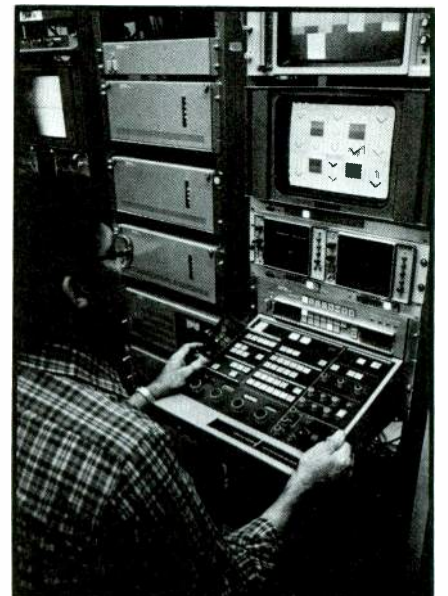
Art Henderson, maintenance technician, shown at the SCU, checks the registration of one SK-110 camera.
