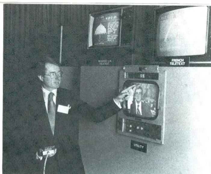
John McKay , KMOX-TV vice president and general manager, points to teletext data in the vertical interval of the program signal. Receivers at the top left and right show actual teletext page information. McKay is holding the keypad controller for the French Antiope system.
