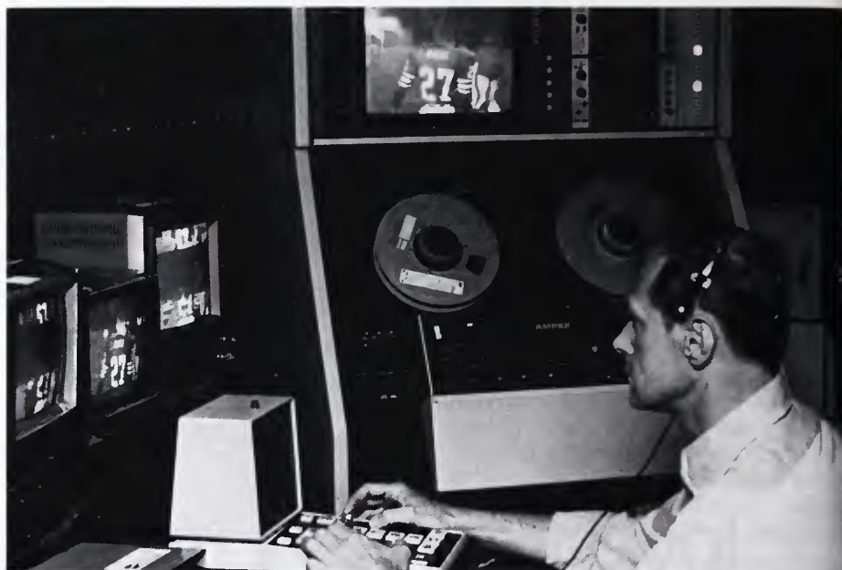
ABC Sports used 2 Ampex VPR-2 VTRs for instant replay/slow motion during a recent Monday night football game. It was network TV's first use of Type C for slow motion and of the SMC-60 slow motion controller.
