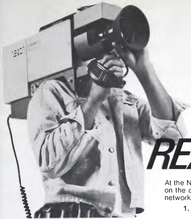
ACC-2000 Portable Color Camera —TV camera hand-held on remote or tri-pod held in studio. Center of gravity conforms to human head, shoulder, arm and hand. Fights fatigue.
