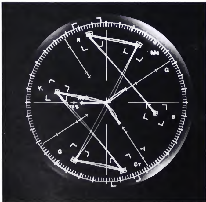
This is the vectorscope reading for the color bars in Ampex's demonstration experimental digital VTR.
