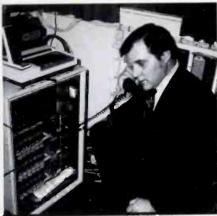
The author Eric Landau, Motorola market sales manager, monitors comparator output on one of three Spectra-TAC receiver voting systems in the teletype room at ABC News, New York City.
