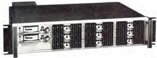
D-501 Audio Distribution Amplifier , 6 outputs, +24 dBm, up to nine D.A.'s with redundant common P.S. in 3 1/2" rack frame
