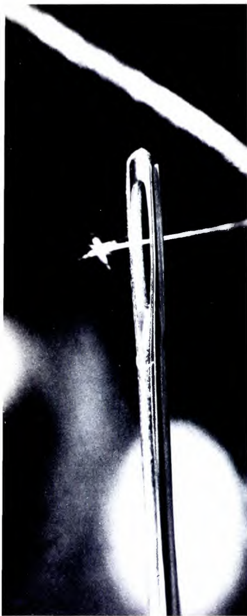
Figure 2 A standard-size sewing needle is used to illustrate the extremely small size of a piece of optical fiber. The fiber is 90 microns thick, which is about the size of a human hair. (Photo by Ron Whittaker).
