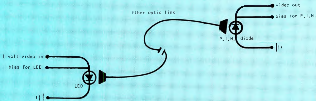
Fig. 1 The basic concept for an optical fiber (OF) system is illustrated here. Even with today's limited OF technology, it is estimated that it is possible to send video signals six to nine miles before re-amplification is necessary. No frequency equalization or AGC processing is necessary.
