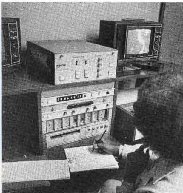
After returning to the newsroom, the reporter plays back the news story and records a time code on the tape. The time code makes it possible to recall important segments without again viewing the entire tape.
