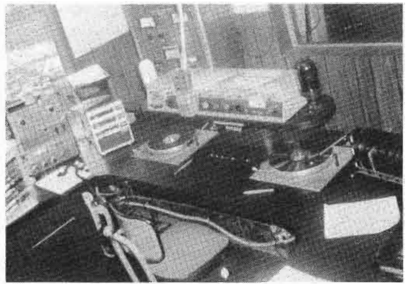
Fig. 7 KENE is another station with the turntables under the board. But since this is not a standup operation, the turntables are pulled out enough to allow easy access and elbow room. The raised board allows easy turntable operation and does not require extra lighting.
