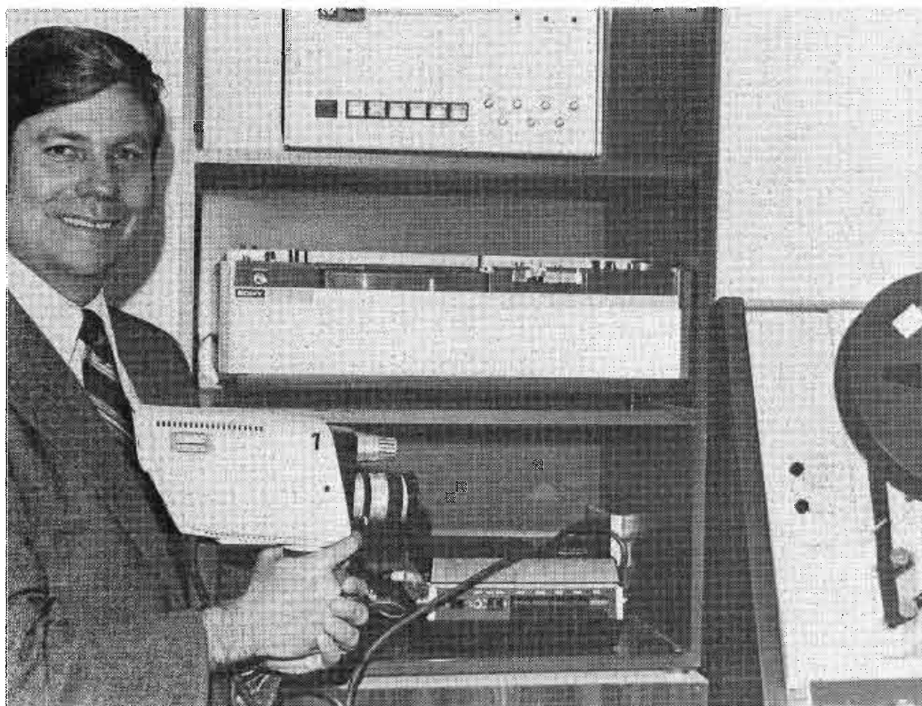
Fig. 1 Dick Fletcher of CVS holds an Akai color camera connected to a portable recorder—one of the economy approaches to electronic journalism. Doubtless, competition to gain dominance in the portable market will bring on even smaller and lighter models. (Photo by Donna Roizen)
