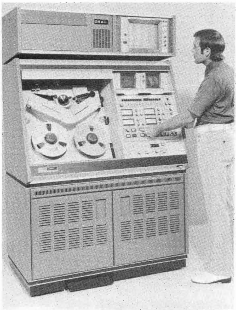
Fig. 6 This is the IVC broadcast quality helical recorder that has drawn so much attention.
