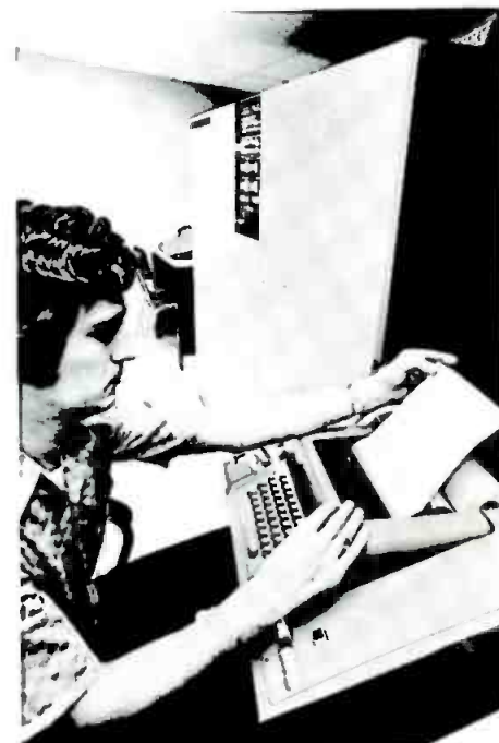
The teleprinter linked to the System/7 automatically logs any values that go out of limits and the time they are brought back within limits. It prints the FCC log every half-hour.
