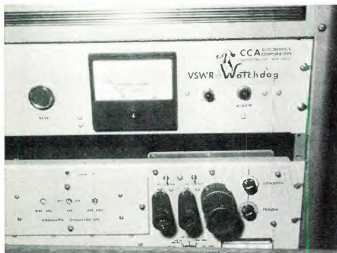
The sentry unit should be a vital protection unit in your system. This unit, called the "Watchdog", is shown in the rack at WLBC.
