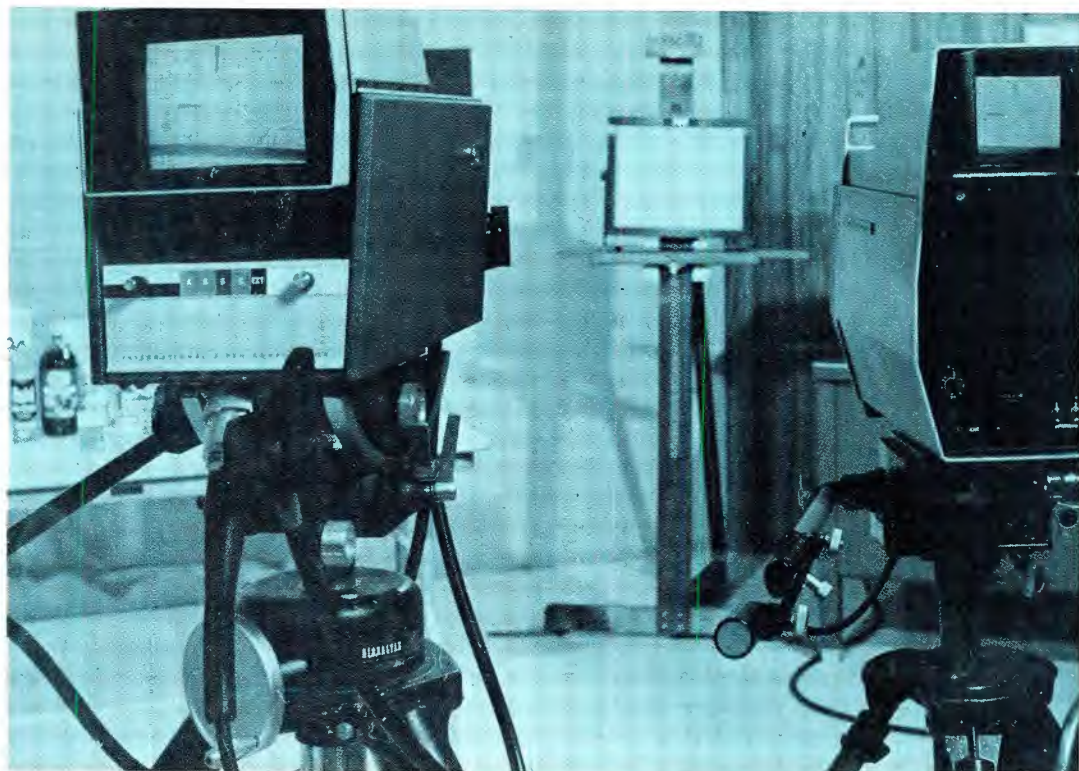
Fig. 1 Here you see two cameras being tested and compared. Note that first set up against a test pattern. Then they will be pointed at a test scene.
