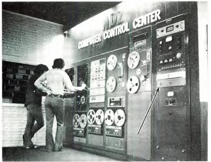
The arrow points to the Wdz impatient listener alarm. Such alarms are vital to automated stations.
