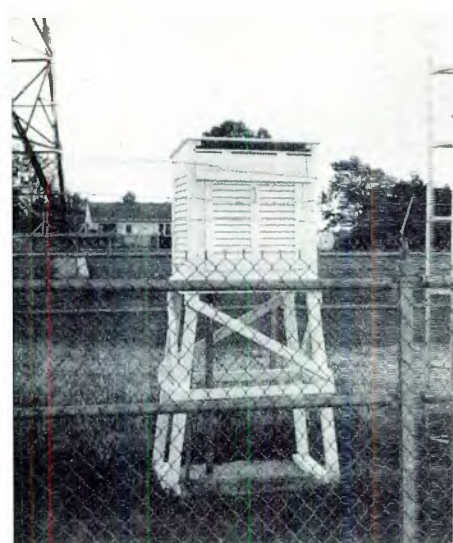
Outdoor weather housing for weather instruments in use at WLBC in Muncie, Ind. Sensor for electronic thermometer is housed here also. All cables run through an underground conduit.
