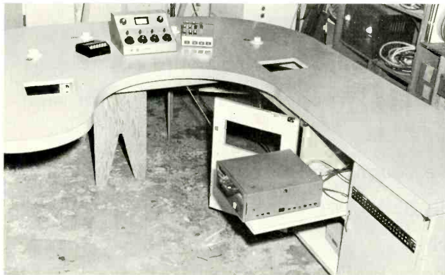
Fig. 5 The WTAQ design allows full access to the cart machine via the cutout in the panel door and the sliding drawer.
