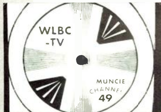
Fig. 7 Photo of test pattern taken off monitor. This is a picture of the waveform with video information displayed in Figure 6.
