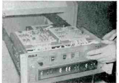
Top: Shibaden's 3-tube color camera and some local scenery. Middle and below: Tape Editing Programmer by RCA has guts housed in compact slide-out drawer, uses 250 flat-pack integrated circuits.
