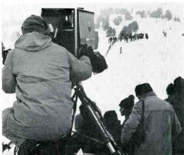
Chained down to wooden platform for easy helicopter lifting, General Electric color camera with directional mic up front, captures action on the slalom.
