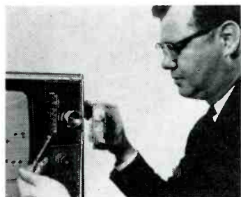
Eugene Walding, engineer section manager for Oak Manufacturing Company's Advance Tuner Development Laboratory, points to new three-band continuous tune TV dial on working television equipped with the company's newly-developed all-channel "Mark IV" tuner. Center portion of large control is bandswitch; outer rim (normally "fine tuning") serves as channel selector. In Walding's right hand is the Mark IV tuner, positioned approximately as it is installed in TV receiver.
