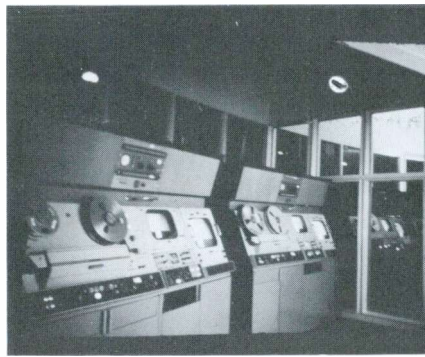
Shown here are two of center's four video tape recorders in the VTR room.
