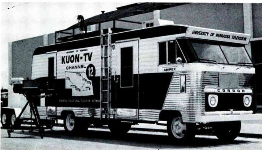
Fig. 1. Specially built van houses mobile unit; power plant is in trailer.
