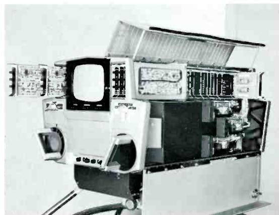
Plug-in transistorized modules speed servicing, increase reliability.
