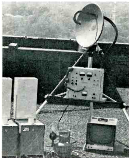
Fig. 3. Microwave link using TE power.
