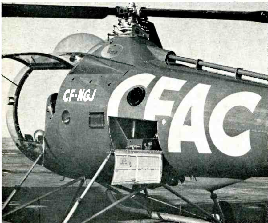
Fig. 1. Brantley B2 helicopter showing location of the equipment for remote use.
